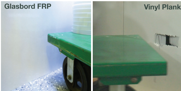
IMPACT RESISTANCE WALL TEST WITH FLATBED CART
