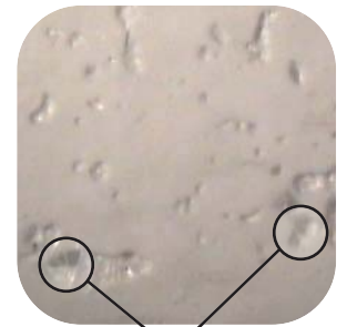
Thermoplastic with a porous surface which can trap dirt and moisture
